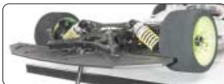
**9.2** Adjust the preload on the rear springs until both front wheels lift at the same time. If, for example, the front right wheel lifts earlier, you must increase the preload on the rear left spring, and decrease the preload on the rear right spring. You must adjust both rear springs, otherwise you will change the ride height.
