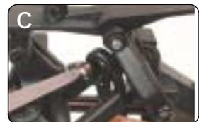
*Remark:* it is not necessary to remove the shocks, however you must be sure that they are long enough not to limit the suspension. Be sure the suspension is reaching the downstop limits, before the shocks do.
