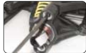
Set the front track-width to 254mm. Turn both pivot balls IN equally to reduce track-width, turn them both OUT equally to increase track-width.
