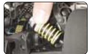
**9.3** Reconnect the rear anti-roll bar, and check for tweak again by lifting the front end of the car. If again one front wheel lifts before the other, the rear anti-roll bar is tweaked. Adjust the length of one or both rear anti-roll bar pushrods until both front wheels lift at the same time.
