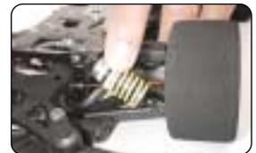
**9.6** Reconnect the front anti-roll bar, and check for tweak again by lifting the rear end of the car. If again one rear wheel lifts before the other, the front anti-roll bar is tweaked. Loosen the screw on the left front anti-roll bar mount. Adjust the eccentric cam until both rear wheels lift from the ground at the same time. Tighten the screw to secure the adjusting cam.
