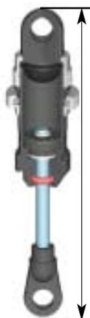
Shock length adjustment: Check the length of the shocks, adjust with the ball-joint.
