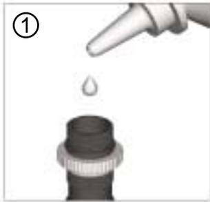
Fill the cylinder with shock oil, with the piston in the bottom position.
