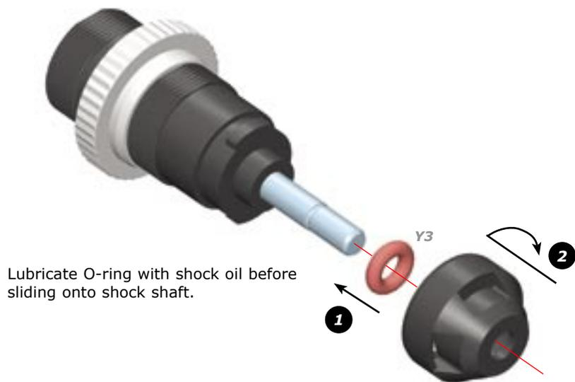
Lubricate O-ring with shock oil before sliding onto shock shaft.
