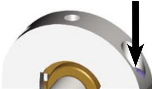
Screw OUT both adjusting screws to shift EARLIER.
