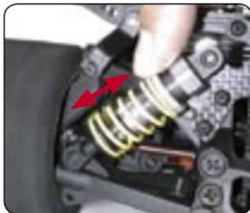
Example: If the front right wheel lifts first, increase the preload on the rear left spring, and decrease the preload on the rear right spring by an equal but opposite amount.
