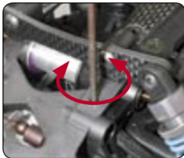
Adjust front downstops by turning the front downstop setscrews into or out of the front bulkheads.
