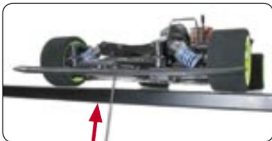
**A10.3** Adjust the preload on the rear springs until both front wheels lift at the same time.
