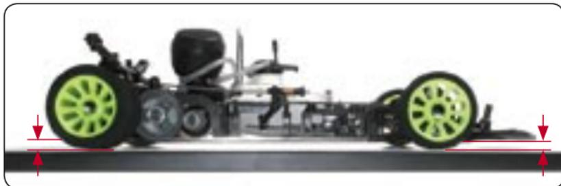
Ride height is the height of the chassis in relation to the surface it is resting on, with the car ready to run. Ride height affects the car's grip since it alters the car's center-of-gravity (CG) and roll center (RC). Because of changes in suspension geometry and ground clearance, there are negative consequences to altering ride height too much.
