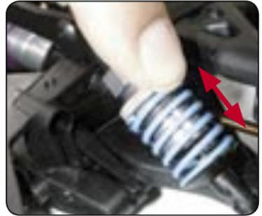
Example: If the rear right wheel lifts first, increase the preload on the front left spring, and decrease the preload on the front right spring by an equal but opposite amount.
