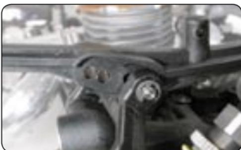
The rear body mount on the Serpent 960 may be connected in several different ways to increase or decrease the downforce transmitted from the body to the rear wheels.
