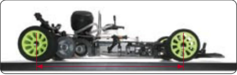
Wheelbase refers to the horizontal distance between the front and rear axles. Changes to wheelbase can have a dramatic effect on the handling of your car, since it re-adjusts the distribution of weight on the wheels (which adjusts grip).
