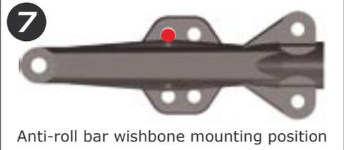
Anti-roll bar wishbone mounting position
