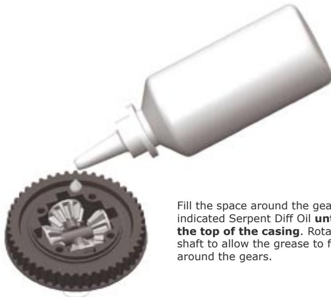
Fill the space around the gears with the indicated Serpent Diff Oil **until level with the top of the casing**. Rotate the output shaft to allow the grease to fill all gaps in and around the gears.
