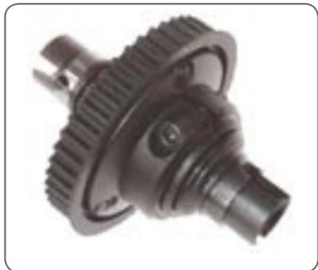
The rear differential can be combined with all types of front axles. The advantage of the rear ball differential is that it can be quickly adjusted to adapt the Serpent 720 to varied track conditions, using a single screw. Drawbacks include the possibility of diff slippage if the internal adjustment screw is not sufficiently tight, and also that running an excessively loose diff action (when slippage is tight) will result in rear end looseness if one wheel starts spinning.
