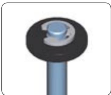
Damping mainly has an effect on how the car behaves on bumps and how it reacts initially to steering, braking, and acceleration. Damping only comes into play when the suspension is moving (either vertical wheel or chassis movement or due to chassis roll), and loses its effect when the suspension has reached a stable position. Without damping, the shock springs would cause the shock to "pogo" or "bounce" (compressing and rebounding) until it stabilized.
