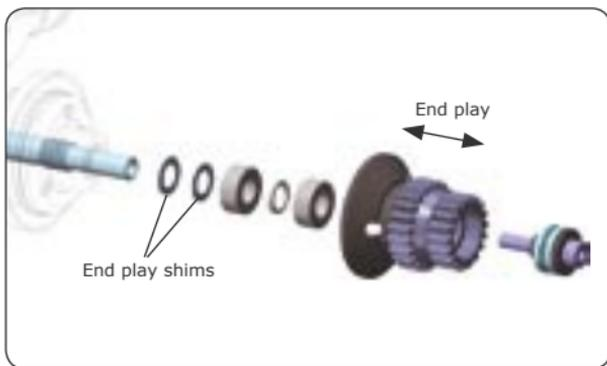
Clutch housing end play is the amount that the clutch housing moves along the crankshaft.
