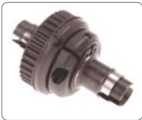
Using the front differential combines some of the braking advantages of a solid front axle while allowing inner/outer wheel speed difference. This last adjustment depends on how much friction is applied with the external friction collar.
