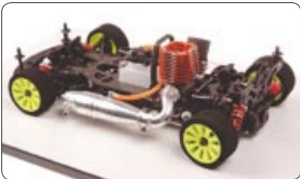
A "roll center" is a theoretical point around which the chassis rolls, and is determined by the design of the suspension. Front and rear suspensions normally have different roll centers. The "roll axis" is the imaginary line between the front and rear roll centers. In general, a higher roll center on one end of the car creates more weight transfer at
