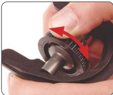
The S400 features a ball differential in the rear and a solid axle (spool) in the front. Optional available is a front differential as well as a one way axle.
