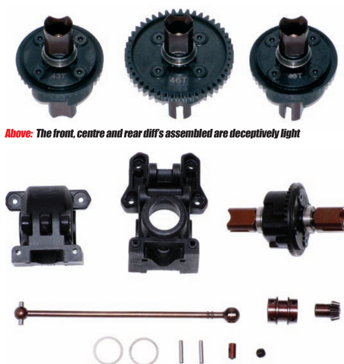
Above: Rear gearbox and drive axle components laid bare...
