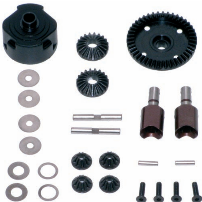
Above: Front diff assembly ready for the build
