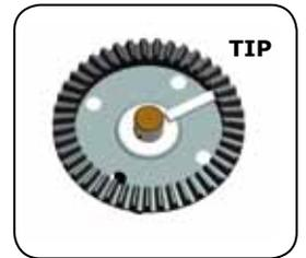
**Differential oil cst value:** compared to the previous diff-gears, you need to use 2.000cst heavier oil as starting point.
