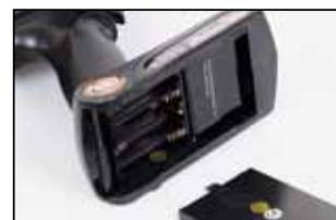
Remove the battery cover and put in 4 AA size batteries.
