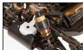
Front anti roll-bar
