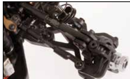
Wheel-axles and driveshaft front
