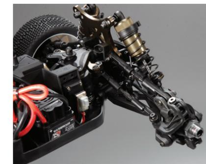
Up front, the camber and toe can be adjusted via the thick steel tie-rods that screw into the large rod ends. This is what we like to see used for a durable race set-up. The huge bore shocks are great for handling consistency over long runs, but they don't come with dust boots and that can mean more frequent rebuilds.
