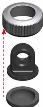
1-Bleed: push the shockrod all the way in slowly, to allow excessive oil to escape.
