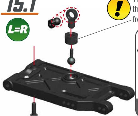
Tighten anti-roll bar cap until there is no play, and it moves freely.
