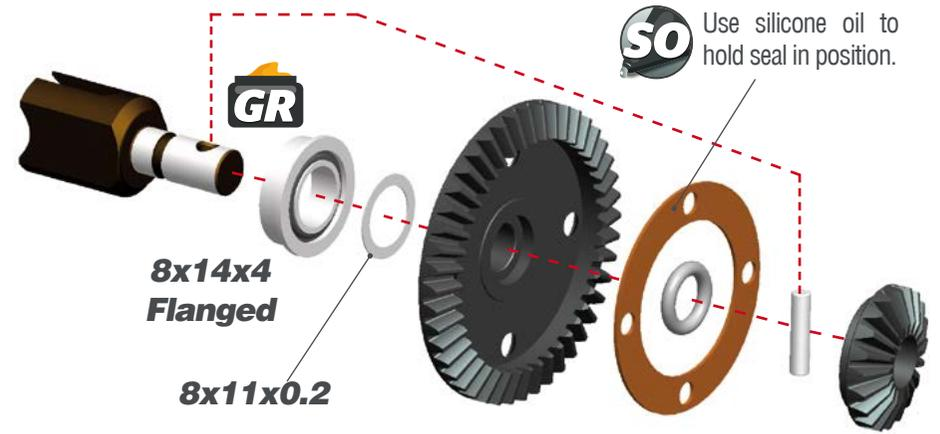
Note the correct way to assemble the pin.
