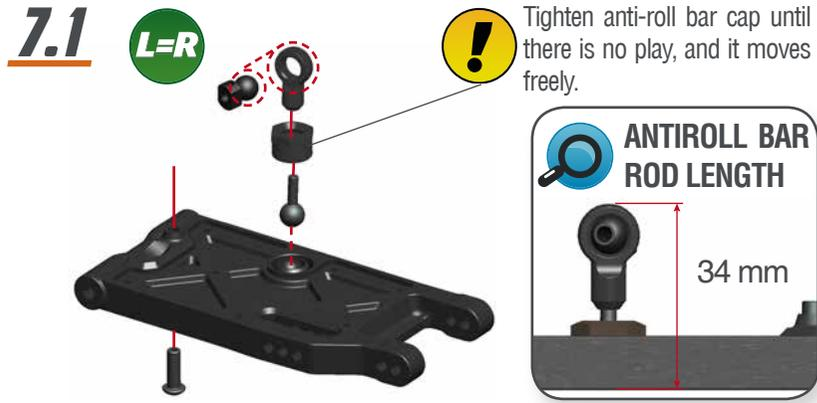
! Tighten anti-roll bar cap until there is no play, and it moves freely.
