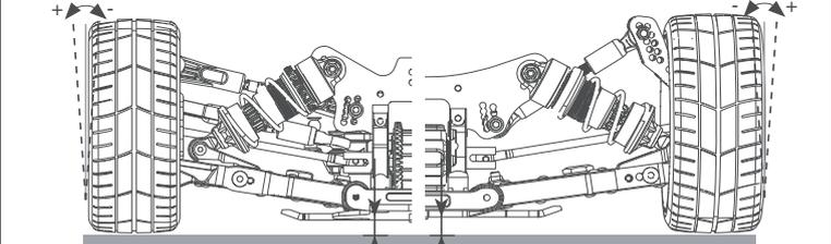
RIDE HEIGHT 8 mm WITH TYRE Ø mm RIDE HEIGHT 9 mm WITH TYRE Ø mm
