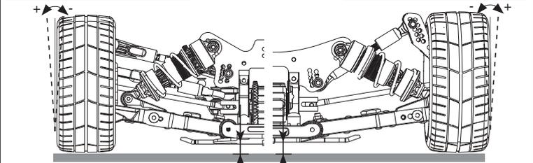
RIDE HEIGHT 9 mm WITH TYRE Ø mm REAR 10 mm WITH TYRE Ø mm
